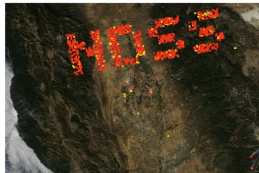
Fig. 1: An overshadowing signal from the attacker manipulates the infrared channels of satellite imagery to create fictitious fires in the resulting dataset.
